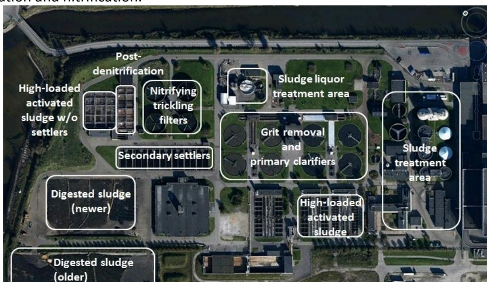
**Figure 1.** An aerial photo of Sjölanda WWTP with marked positions of important process steps.
