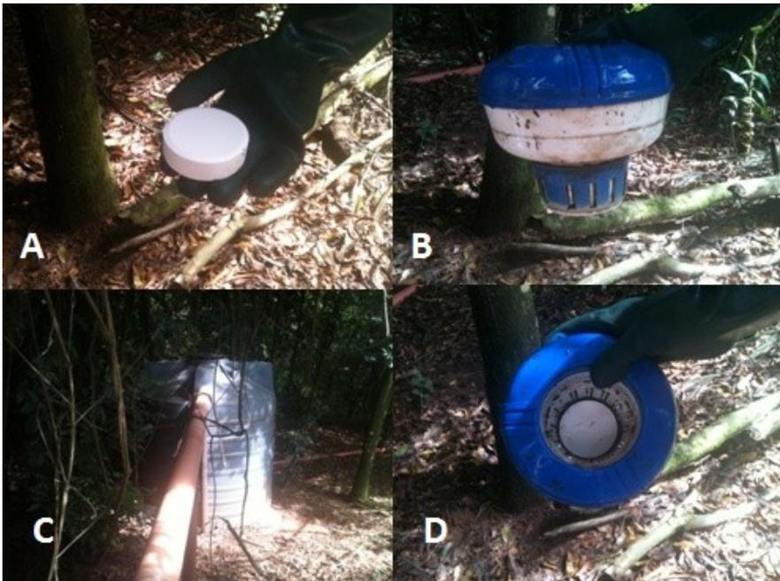
**Figure 2.**(A) A tablet of chlorine, (B and D) floating Chlorinator (C) disinfecting tank.
