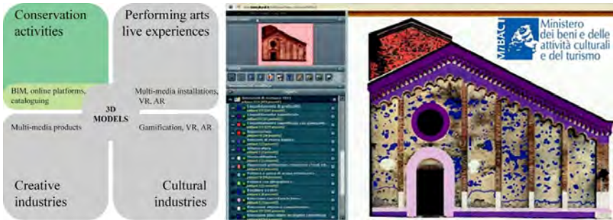
Fig. 3 - SICaRweb, the interface of the system that shows a decay mapping on the elevation of the building (on the right), and its relation with the CCPS system (on the left).
