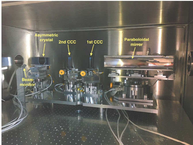
Fig. 3. Optical components for beam handling, positioned on their motorization stages in the optical chamber.
