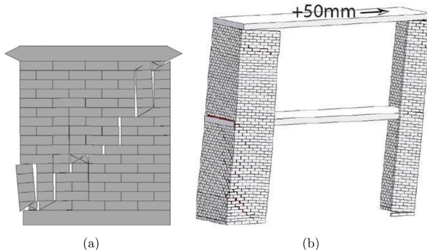
Figure 11: Examples of contact-based approaches which include masonry crushing [100, 49].
