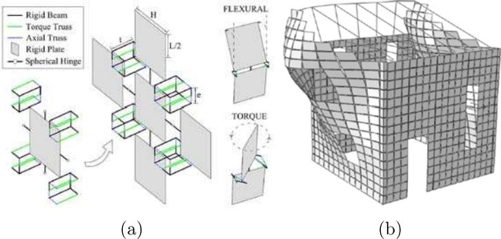
Figure 17: Examples of homogenized RBSM approaches [197, 169].
