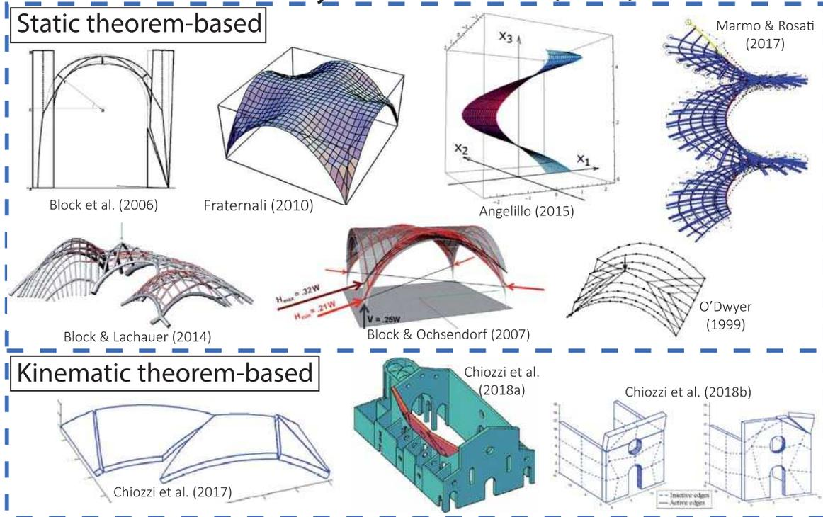
Figure 18: Examples of geometry-based models.
