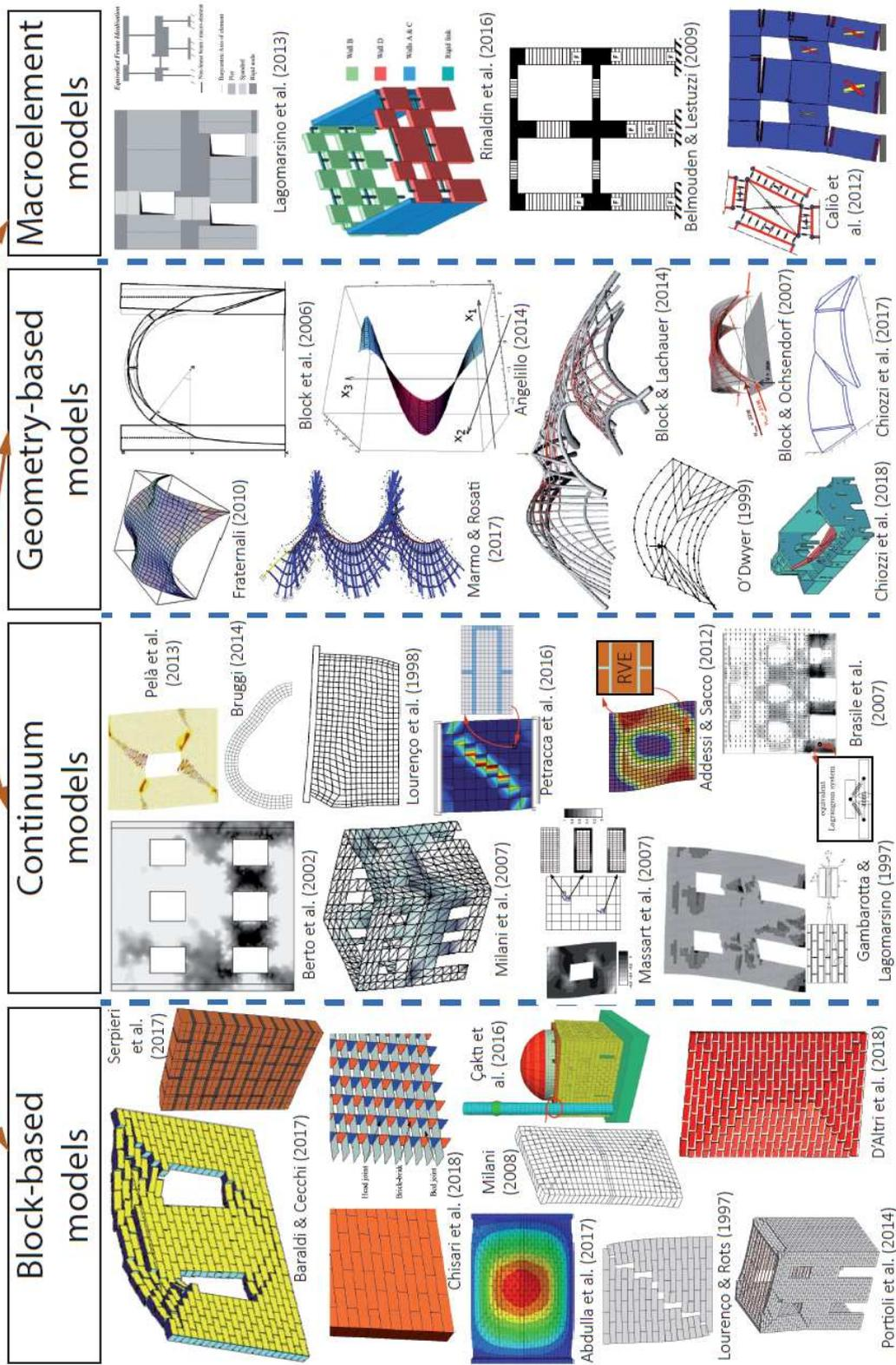
Figure 2: Modeling strategies for masonry structures.
