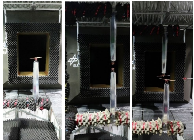
Fig. 1 Experimental setup: single rotor (left), coaxial rotors (middle) and tandem rotors (right)
