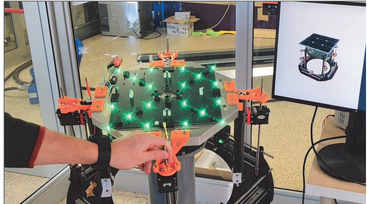
Fig. 7: STASIS Attitude Ground Truth system
