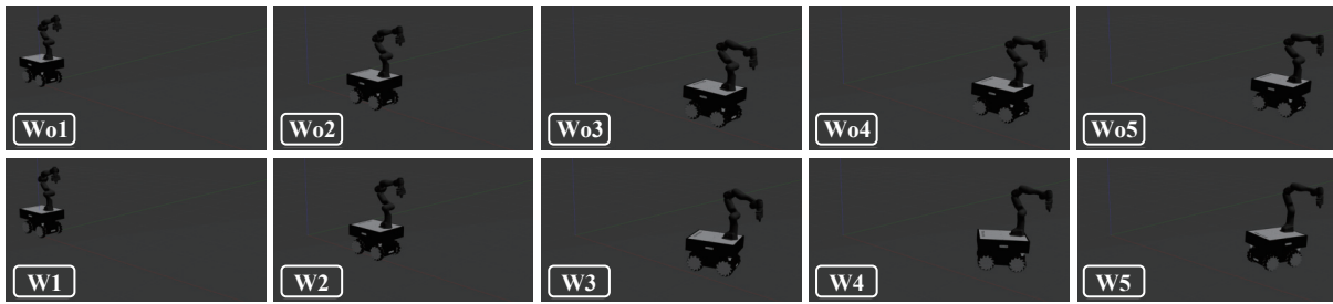
Fig. 4 Snapshots of the ablation experiments in Gazebo. The first row: the proposed approach is without the learned mobile base pose tracking item in the secondary task of HQP. The second row: the overall proposed approach (i.e., with the mobile base tracking item in HQP).
