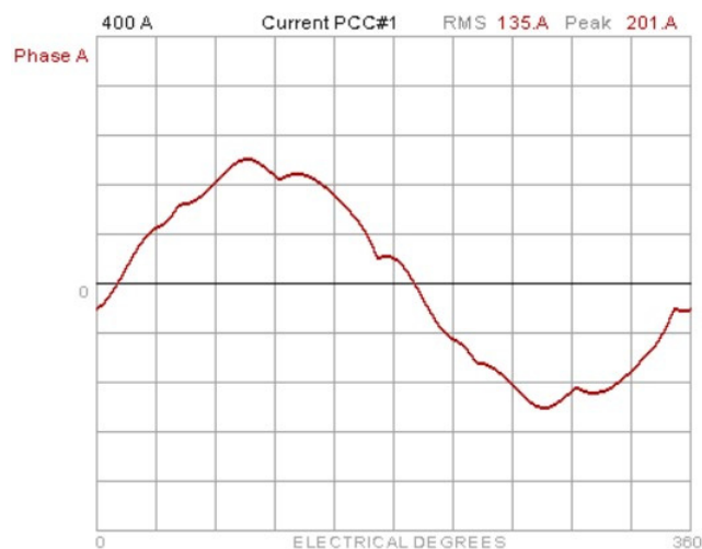
Figure 32. AUHF test result simulation. Phase source current waveform at full load of AUHF-injected current.
