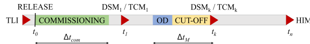
Fig. 5 Time schedule during transfer. The orbit determination and cut-off time intervals are repeated before each maneuver.
