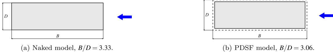
Fig. 4. Quoted sketch of the top view of the model. The blue arrow indicates the wind direction.
