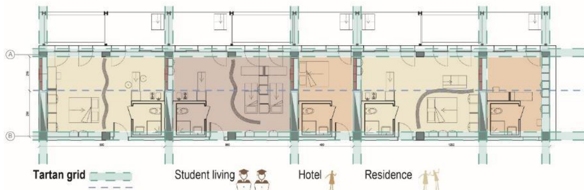
Figure 3. Example of dimensional and modular coordination, Elaboration by Vignati, G., based on an unpublished work by Ceriani, J., Frontera, E., Faldrini, F.
