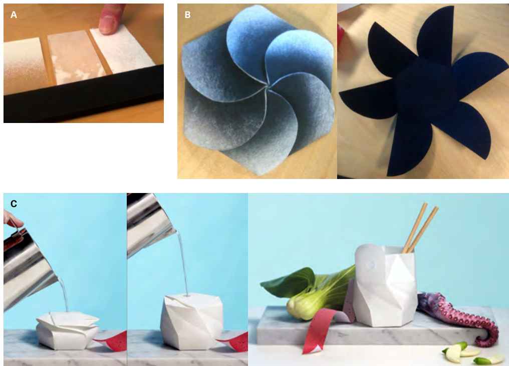
Fig. 2 RISE AB. The material is cellulose-based and developed by RISE. Cellulose-based active material as a) abstract (more technology-driven) demonstrators (swatches) of the material before activation b) conceptual demonstrator as self-opening cone before (left) and after (right) activation c) a (more market-driven) conceptual material demonstrator in the context of a self-expanding packaging used when rehydrating dry foods with hot water.
