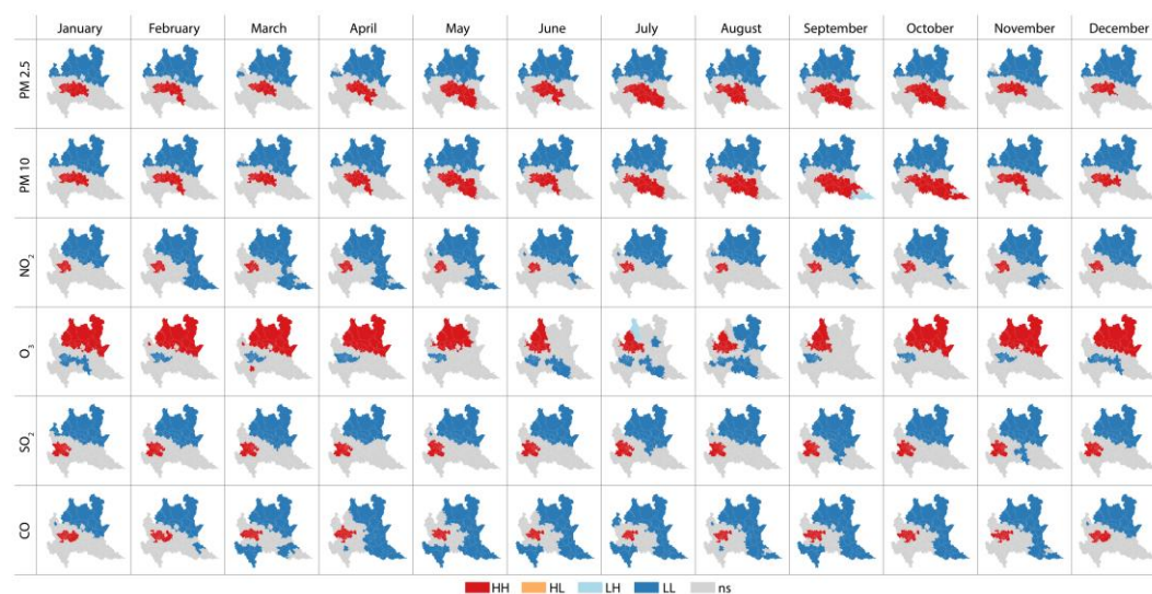
Figure 5. Local Moran's I computed on 96 districts of approximately uniform population of 100,000 residents across the territory of Lombardy region, Italy, for different air pollutants (concentration values reported by Copernicus CAMS reanalysis data). Red and dark blue areas correspond to High-High and Low-Low clusters, respectively, while the remaining areas in grey resulted not significant for clustering purposes.
