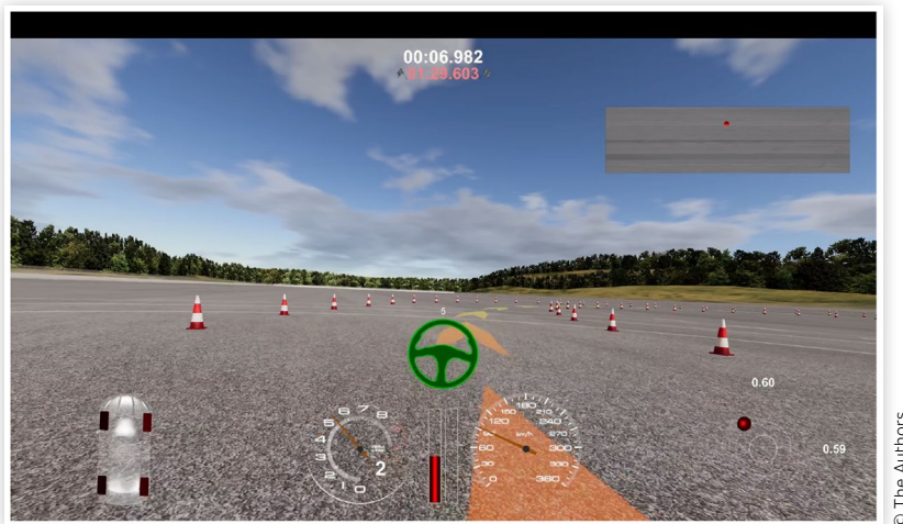
FIGURE 6 Dynamic Simulator view from the driver's perspective with the racing ribbon overlaid on the scene, indicating the desired trajectory to follow.
