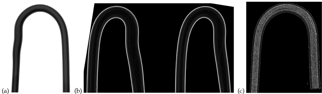
Fig. 7 Black and white detail image of a deposited PP tubes with R/OD=6 (a); details of outer profile of two tubes with R/OD=3 after edge extraction with the software Image J (b); inner profile of a tube with R/OD=6 after edge enhancement (c)
