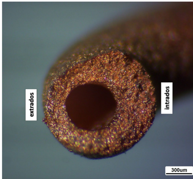
Fig. 19 Cross-section of a sintered tube, extruded with R/OD = 1.25
