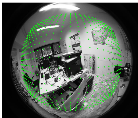
Figure 4. Transformation maps plotted on the fisheye images. The mapped green points are subsampled pixel index, the undistorted image will be generated by aligning them in a regular orthogonal grid.
