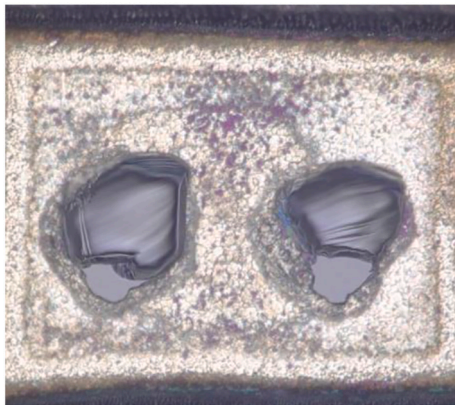
Fig. 11. Ball lift signature of legs with 1 \mu\text{m} -thick bond-pad after being subjected to 200 ^{\circ}\text{C} HTS.
