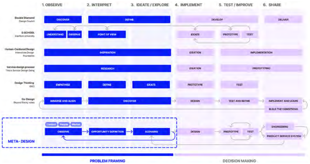
Figure 2. List of design process models inspired by Bravo and Bohemia (2019). Meta-design acts as a problem-framing that is compared with other design processes.
