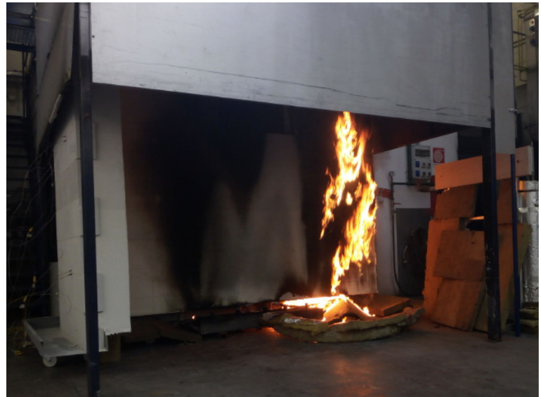
FIGURE 15 Sudden reignition phenomena occurred on the specimen with EPS insulation (test 5 of Tables 2 and 3). EPS, expanded polystyrene [Colour figure can be viewed at wileyonlinelibrary.com ]
