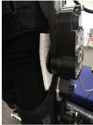
Fig. 3. Example of 3d textile applied as comfortable cushion for exoskeleton joint
