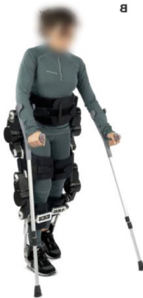
Fig. 1: The exoskeleton Twin without the smart t-shirt
