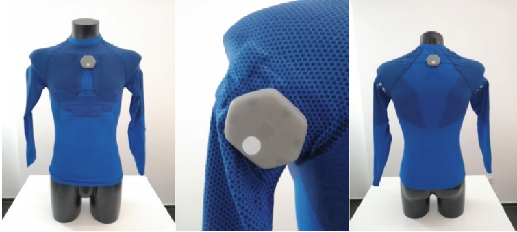
Fig. 4. The sensorised t-shirt. The devices are connected on the back for trapezius EMG, on the arm for deltoids and triceps, and on the front for ECG and respiration measurement.
