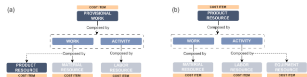
Figure 2. (a) Structure of provisional work and the resources/ product resources that compose it; (b) Structure of the product resources and the resources that compose it
