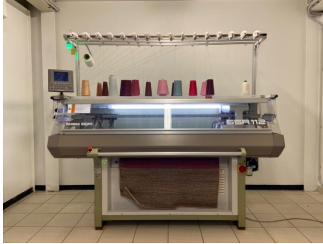
Fig. 2. A CNC knitting machine. The protections prevent the manual intervention of the operator. The entire process is set and controlled remotely.
