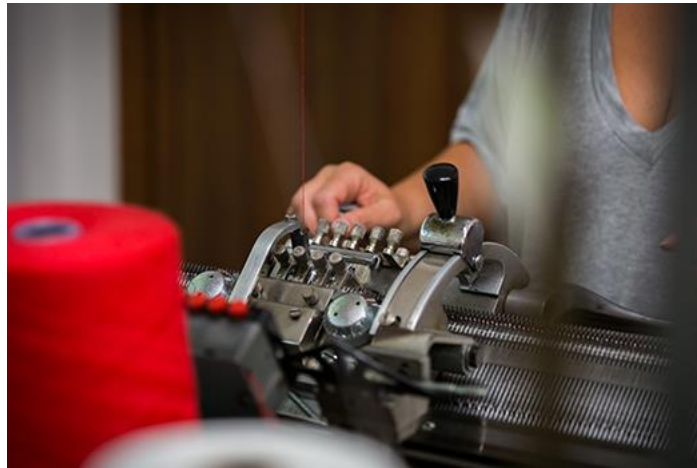
Fig. 1. The carriage of a manual knitting machine diffusely used for production until 1970s, operated by hand.
