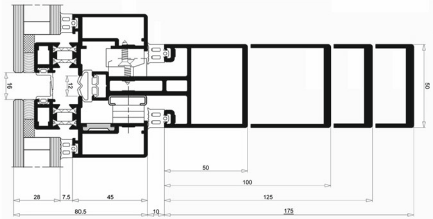
Fig. 3.7 Constitution of the structural system which observes the configuration of the mullion according to the external projection of the double-rib central pivot, with internal transverse stiffening, the lateral application of the frame profiles, with the wing section projecting towards the internal central seal, and the connection of the polyamide bar connectors. © Courtesy of Metra
