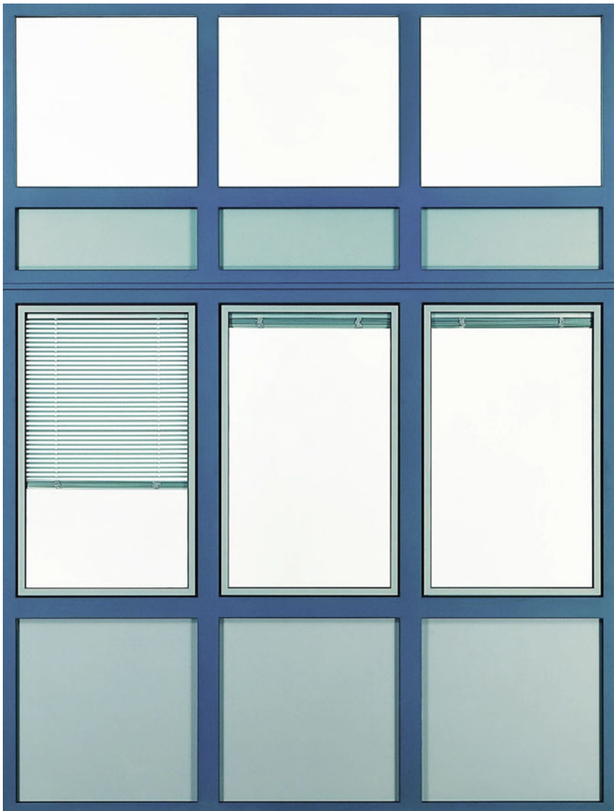
Fig. 2.24 Configuration of the PVC mullion and transom façade typology which observes, specifically, the constitution of monobloc frames, the definition of multi-chamber sections, capable of high thermo-acoustic insulation values and of reducing the formation of surface condensation, and the insertion of galvanized steel coupling reinforcements. © Courtesy of Finstral
