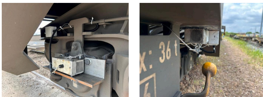
Fig. 14. Cm-scale wind turbine positioning on: (a) Axle-box (b) Lateral underframe of the carbody.
