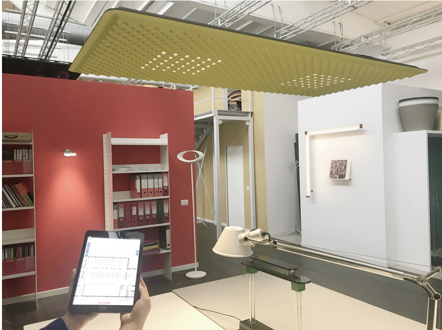
Fig. 5 – The Artemide App makes it possible to gather information through presence and daylight sensors built-in Artemide lamps. This creates Heat Maps in the App that allows the collection of essential data on the behavior of who interacts with space and allows the setting of lighting control parameters. Courtesy Artemide.
