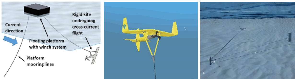
Figure 30: Major components of an ocean kite system [146]; Minesto Deep Green [166]; and SeaCurrent Tidal Kite [167].
