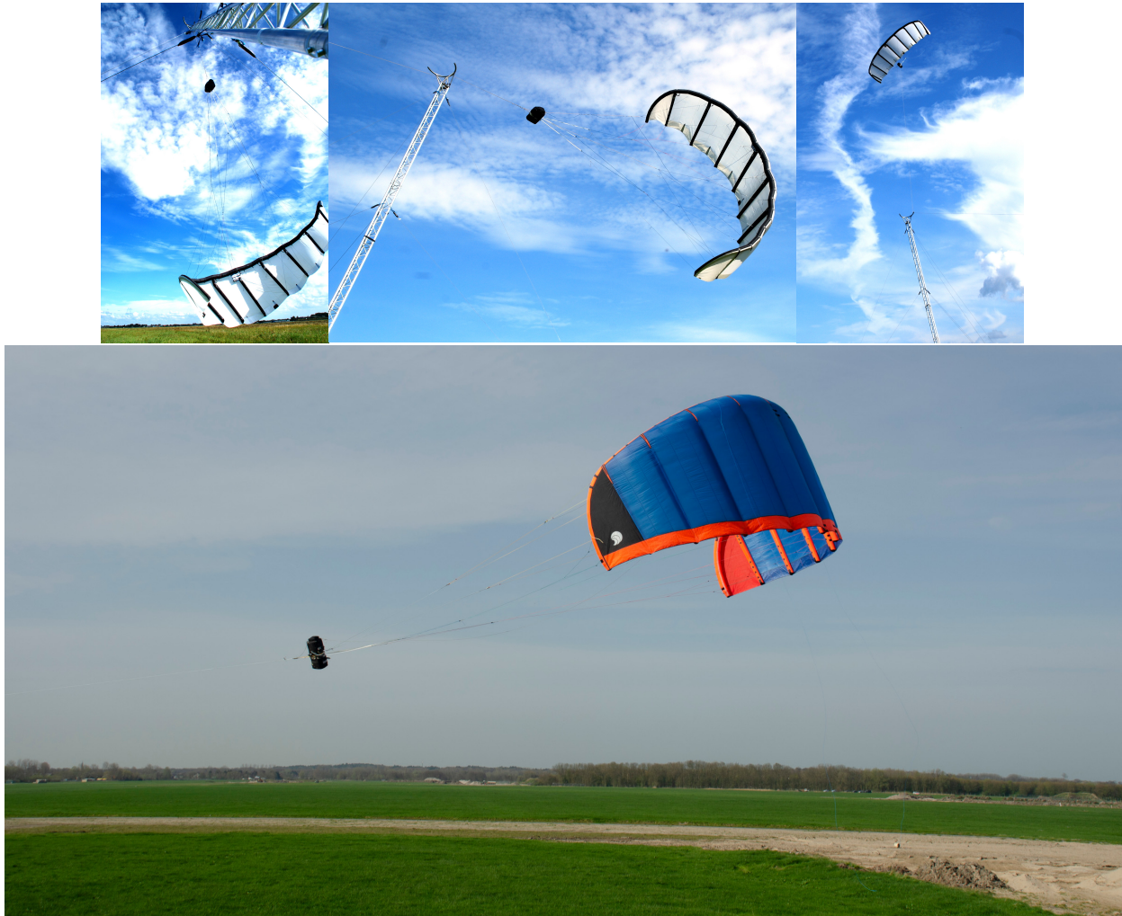
Figure 26: Experimental launch of a 25 m 2 V 3 leading edge inflatable tube kite from an upside-down hanging position on 23 August 2012 (top), standard half-automated winch launch of a 40 m 2 V 5.40 derivate kite, temporarily reaching a tether force of 15 kN and a mechanical power of 100 kW during a test flight in May 2018 (bottom) [147].
