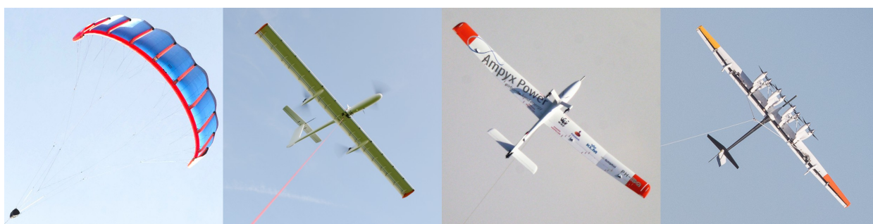
Figure 1: Selected AWE systems currently in development: Kitepower, TwingTec, Ampyx Power and Makani Power (from left to right), generating up to 600 kW per single system (photos from [28]).
