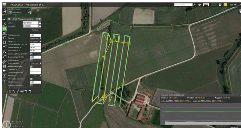
Figure 3. The flight plan for the UAV survey over the investigate rice field.
