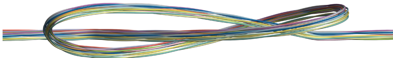
FIGURE 11. Illustration of the bundle with 7 TWPs used for Crosstalk and FWC prediction.
