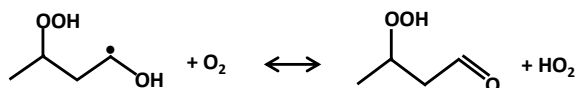
Figure 10. \alpha -Hydroxy-hydroperoxyalkyl radical and its interactions with O_2 to form a carbonyl-hydroperoxide (e.g., hydroperoxy butanal) and HO_2 .
