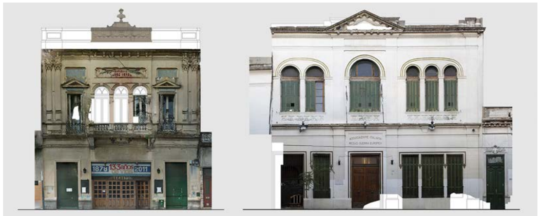
Fig. 7. Facades of Theatre "José Verdi" and Italian Association "Reduci Guerra Europea" processed with Agisoft Photoscan (graphic elaboration by the authors).
