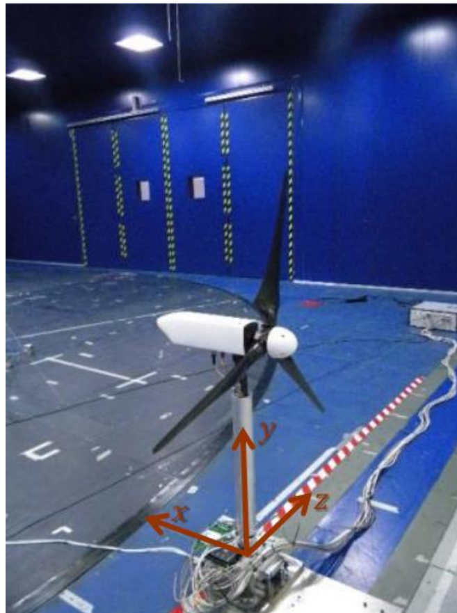
Figure 1: G1 Turbine in Polimi Wind Tunnel (GVPM)
