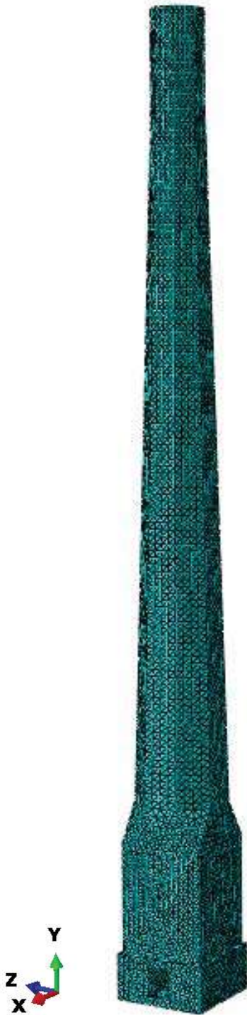
Figure 7: The meshed model .with 3D elements
