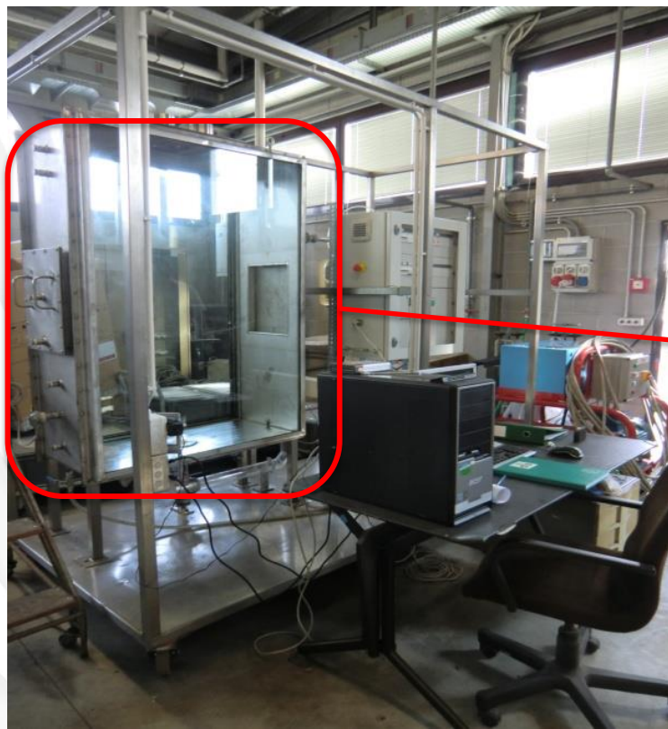
SCRUPOS Facility: SCR ubbing by PO ol and S pray (Layout Pool Scrubbing)
