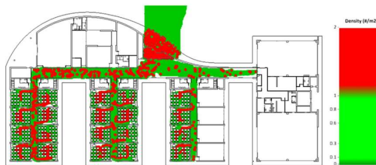
Fig. 3 Density map resulting from crowd simulation on the school of Melzo (one of the two case study buildings used for crowd simulations)
