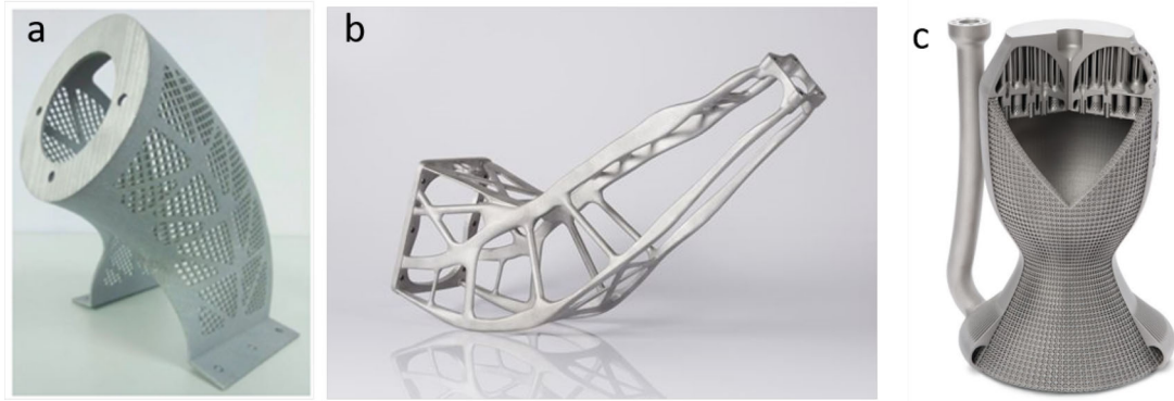
Figure 1. Examples of complex shapes produced via metal AM: (a) lightweight bracket for space applications (Jorge 2018), (b) topologically optimized space antenna support ( https://www.eos.info/case_studies/additive-manufacturing-of-antenna-bracket-for-satellite ) and (c) rocket engine demonstrator ( https://www.etmm-online.com/3d-printing-a-rocket-engine-a-886960/ )
