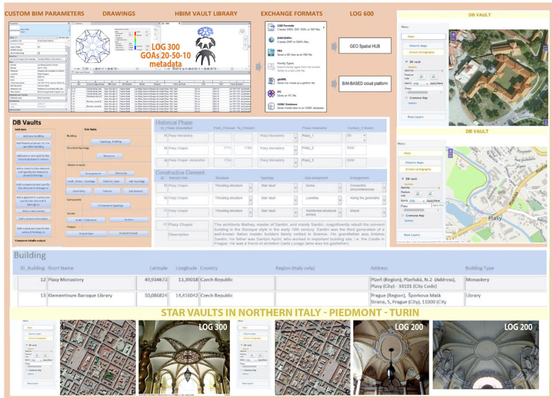
Fig. 14 The HBIM vault library and its exchange formats for LOG 600 through the Geospatial Hub and the BIM-based cloud platform (upper). The GeopanAPP was implemented within the Geospatial Virtual Hub with the Vault GEODB and linked HBIM object libraries. Queries based
