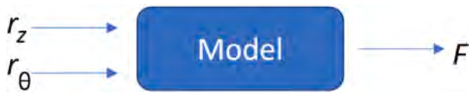
Fig. 2. Identification problem for self-excited force modelling. F could be drag force, lift force or pitching moment.
