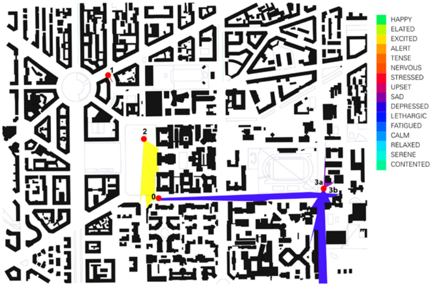
Fig. 5 Clustered PoV. Starting point '3' is duplicated into two different PoVs. The different view-specific partial isovists (field 30°) colored according to the quality of the assessed emotion.
