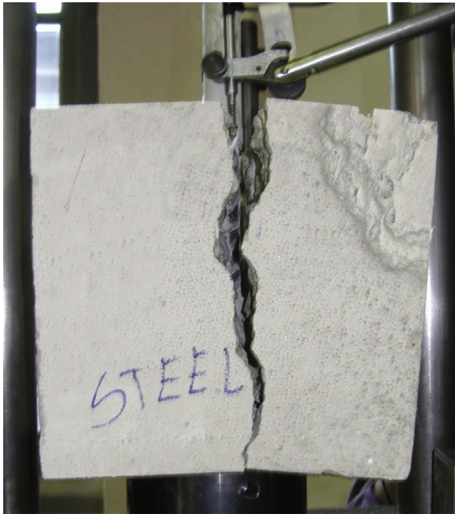
Fig. 8. Failure mode of a specimen with a steel bar of diameter 16 mm.
