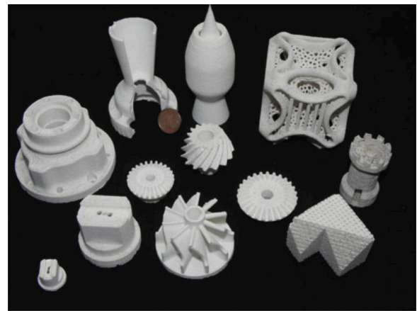
Fig. 5. Pure PBF-LB processed alumina parts manufactured by Juste et al. [25].
