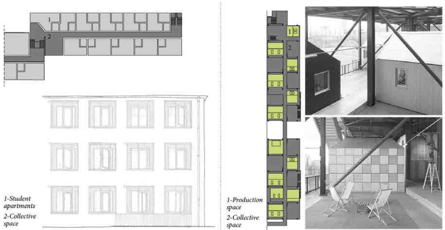
Figure 2. Two adaptive approaches to make the space habitable: reusing the entire building within the envelope (I), exploiting the extant as a support for introducing smaller units (II). Left side: Student Apartment in the former Constable School, Vandkunsten Architects, Copenhagen 2015 (Diagram and sketch: Lepratto 2020). Right side: The Gantry Studios. Architecture 00 + HawkinsBrown, London 2017 (Diagram: Fontanella 2020, photos: Lepratto 2020).
