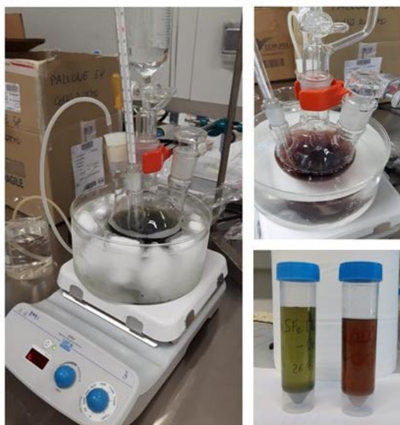
Fig. 3. – Oxidation process at lab scale (1 L); comparison between ferrous and ferric solutions.
