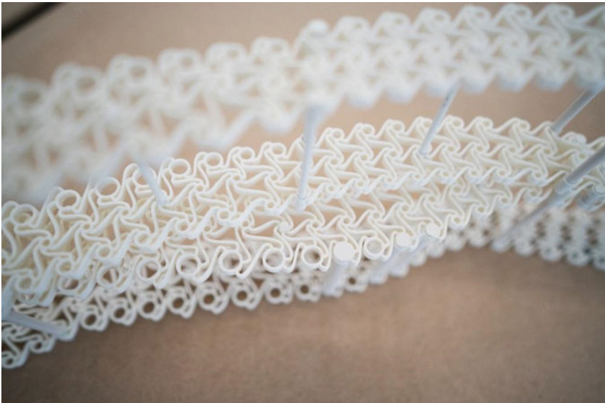
Fig. 6.4 Parametrically designed auxetic pattern used for a shape-shifting wall at Hyperbody, in which a bench is designed to flush with the wall in certain configurations but pop out in others (courtesy of Elpiza Kolo)
