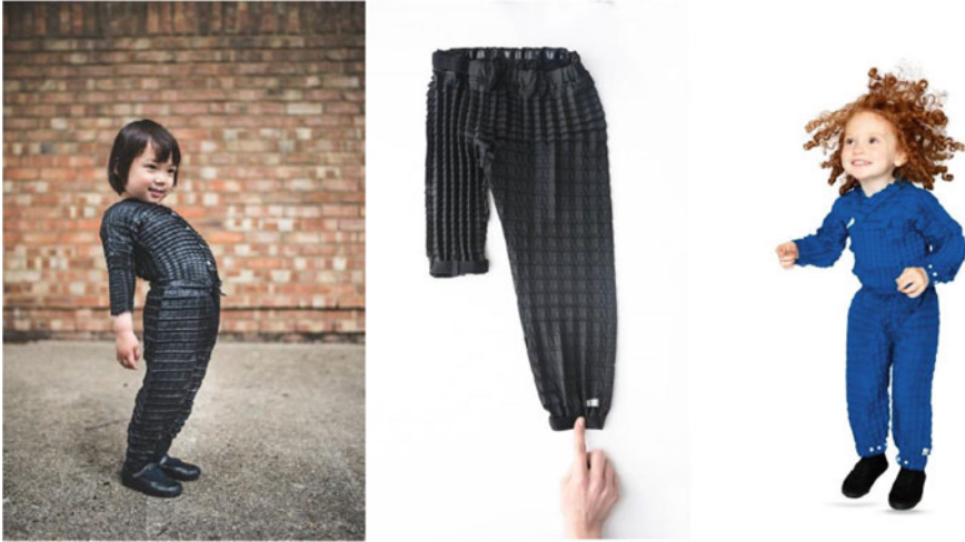
Fig. 6.1 Auxetic materials used by Petit Pli to produce adaptive clothing for kids: the trousers can almost double in size due to the auxetic principle (courtesy of Petit Pli, photo credits: Ryan Mario Yasin, Mollie Rose)
