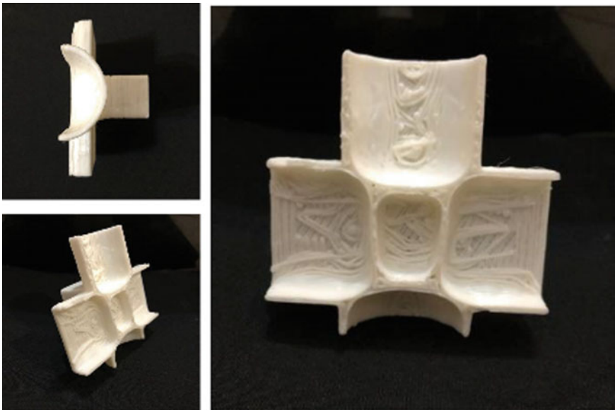
Fig. 4.1 Section of Topology Optimized steel joint prototyped using PLA 3D printing. Image courtesy of Politecnico di Milano graduate research
