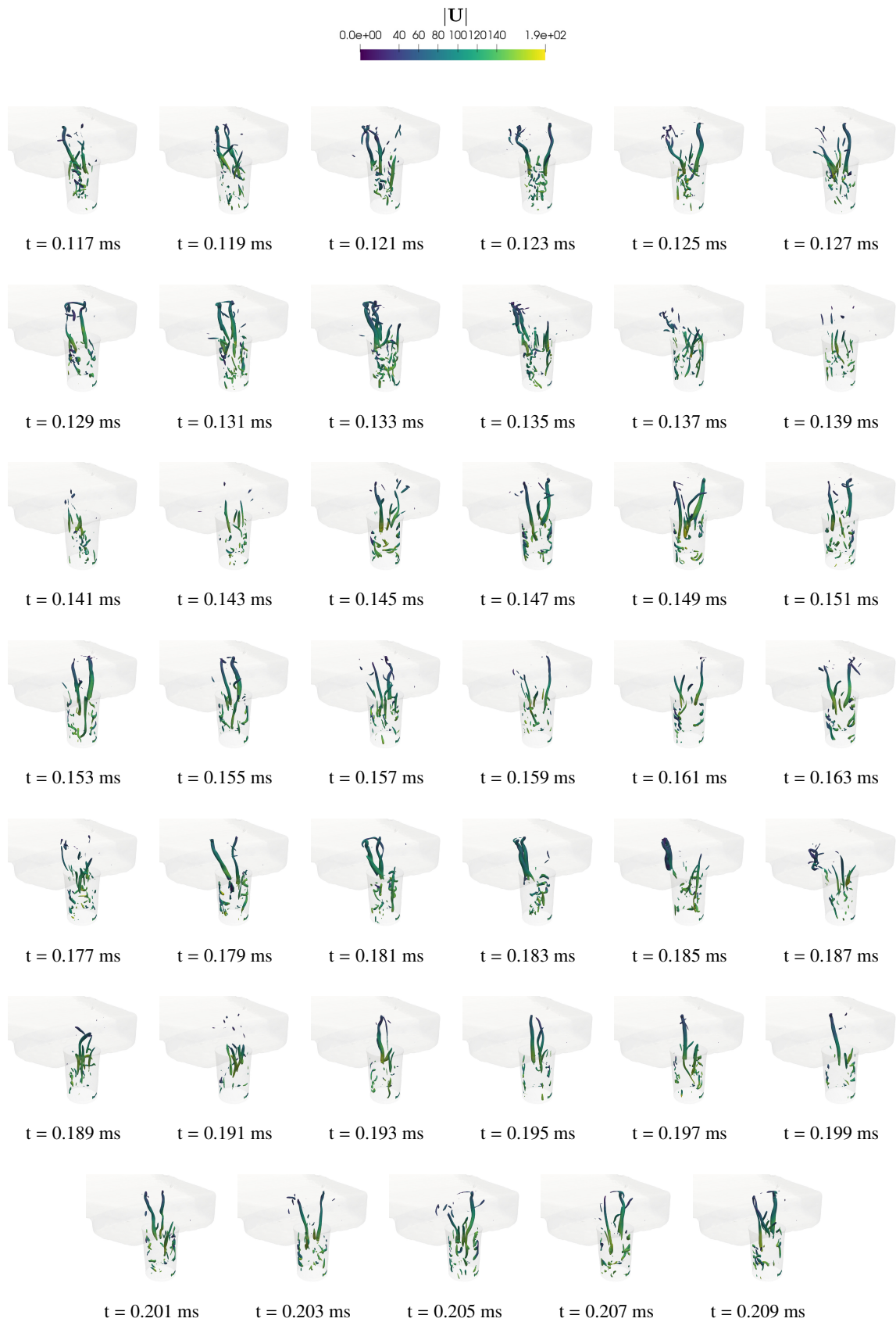
Figure 23: Isosurfaces of the second invariant of the rate of deformation tensor (Q-criterion), showing the evolution of the vortex strings into the nozzle of injector configuration ID-10 during cavitation.
