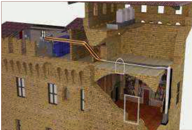
Fig. 1. View of the Northern tower with the main components of the HVAC system.
