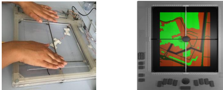
Fig. 1 Model of the F2T (left) and its current prototype (right): a flat thumbstick (center of the tablet) acquires user's intended movements; the actuated support moves the thumbstick to generate a large variety of haptic effects from images displayed on a screen to which the F2T is attached.
