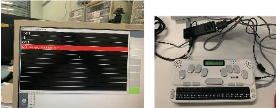
Figure 4 Braille display shows red line messages show in left image. Braille user can read each message on the chat where he wants to access anytime. Also, others can detect these situations.
