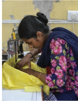
Artisan sewing Monsoon coat out of saris bonded with a film as waterproof treatment.
