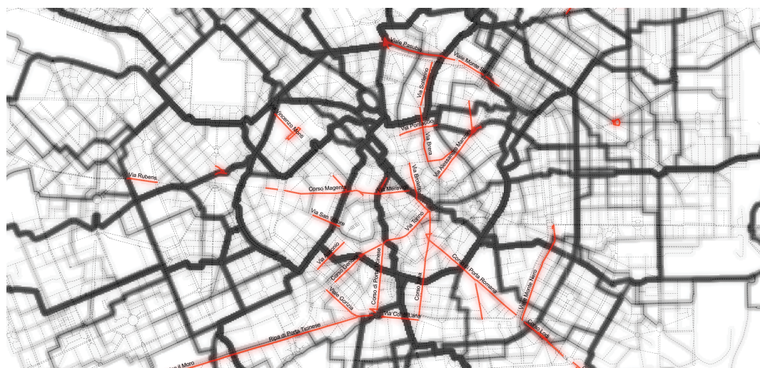
Fig. 4 - Assessment of high impact infrastructural actions. Highlighted in red are high-connectivity roads that are systematically avoided by cyclists due to inadequate conditions.
