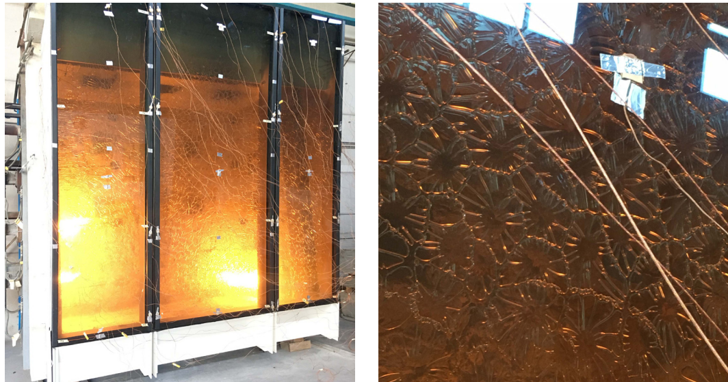
FIG. 26 Façade mock-up under fire exposure (on the left). Glass interlayer appearance after the laboratory test (on the right)
