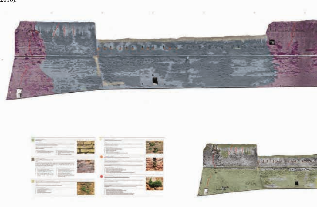
Figg. 17, 18 | Stratigraphic survey of the North facade of the Castle; Decay survey and maintenance project of South-North facade of the Castle (credits: Politecnico di Milano, DASTU and ABC Departments, F. Albani, M. Gambaro, 2018).
