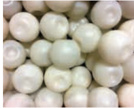
Fig. 5 | BASF's Micronal phase-change microcapsules enhanced gypsum board (credit: materialdistrict.com/material/micronal-pcm/).
