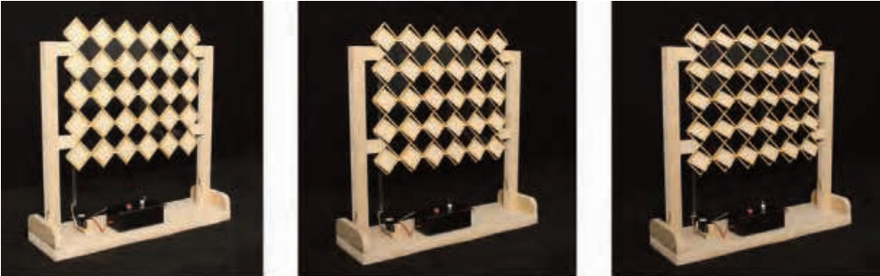
Fig. 4 | Adaptive Sola Skin, self-supporting solar collection façade: prototype with removable panel (credits: danielraznick.com/about/adaptive-solar-skin/ ).
